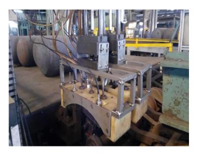
The Seamless Cylinder test systems is to test the defcets Longitudianally & Transverse oriented defects & Wall thickness measurement based on the International Standard. The Test Mechnism will have Bubbler Probe Mechanism for the defects oriented longitudinal, transverse & wall thickness.
